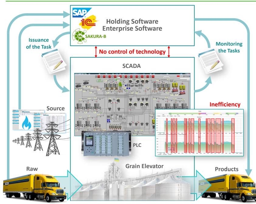
Currently, most elevators in Ukraine have SKADA, which are disconnected from production management and resource control systems. As a rule, automated transfer of tasks and control of their execution are absent. The SKADA operator, guided by its own experience, chooses a technological route from dozens of possible alternatives. Adjustment of technological timings depending on the quality and quantity of raw materials is not applied.
