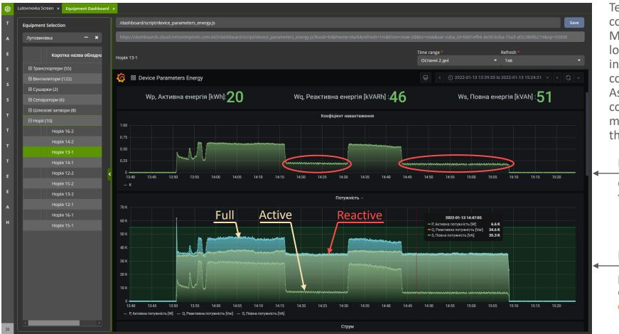
Test operation showed that more than 17% of the company's equipment was used inefficiently. Moreover, if electric motors were idling without load, the energy consumed by them dropped insignificantly. The reason is the high reactive component of energy consumption.
