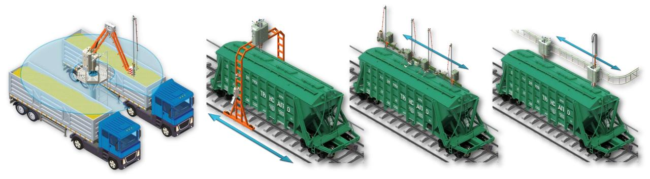
**INNOVINNPROM** sampling systems are designed for sampling of grain crops from car bodies and railway hopper cars and their subsequent transportation to laboratories for analysis.
