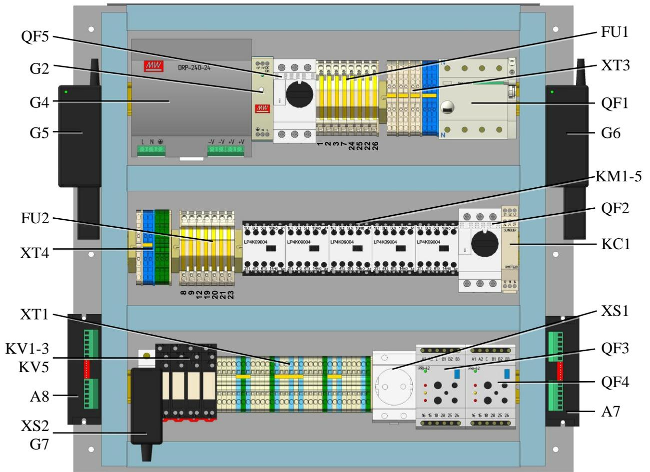
Fig. 3.9. The arrangement of equipment on the rear mounting plate:
