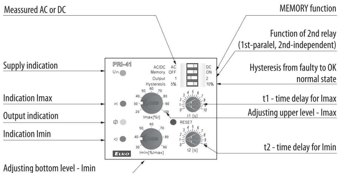
Fig. 3.10. Controls of current monitoring relay ELKO PRI-42
